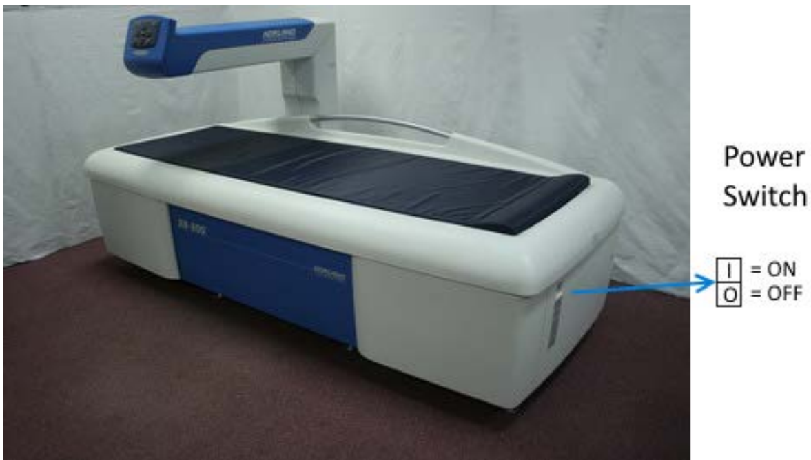
Figure 1-1: Power Switch location
