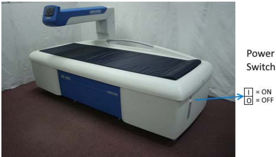
Figure 1-1: Power Switch location
