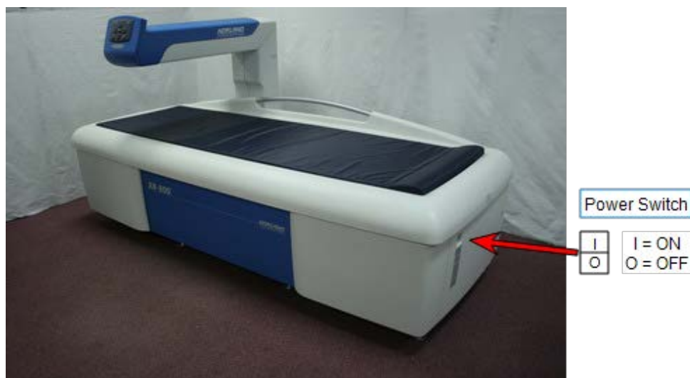
Figure 4-16: Power Switch location
