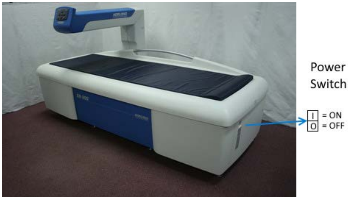
Figure 1-1: Power Switch location
