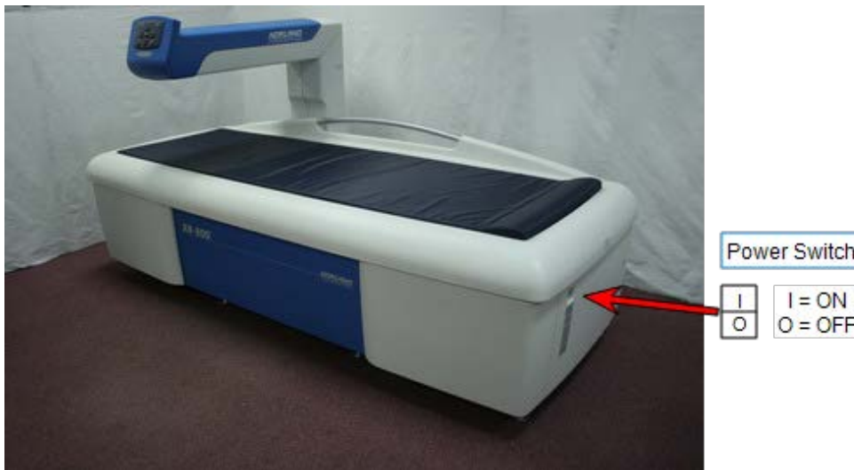
Figure 4-16: Power Switch location
