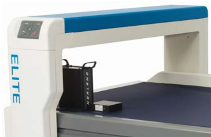
Figure 4-6: Positioning the QA Calibration Standard and QC Phantom
