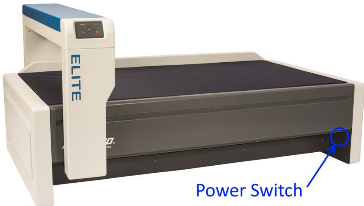
Figure 4-1: Scanner Table Power Switch Location
